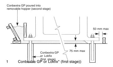
2 Conbextra GP poured or pumped into removable hopper (second stage)
